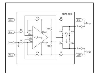
Figure 1. THAT 1646 Equivalent Circuit Diagram
