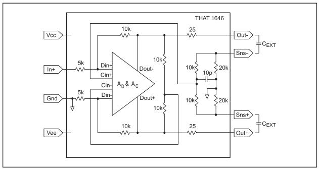
Figure 2. THAT 1646 Equivalent Circuit Diagram
