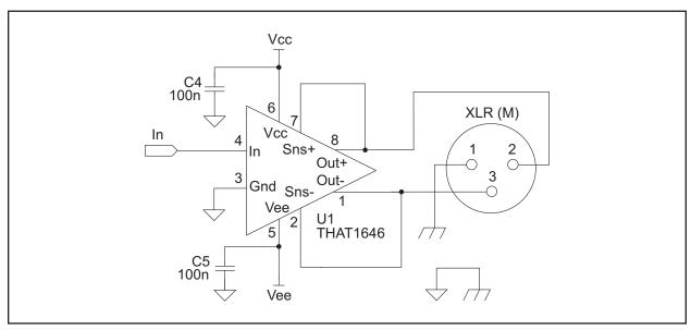
Figure 4. Basic THAT 1646 application circuit
